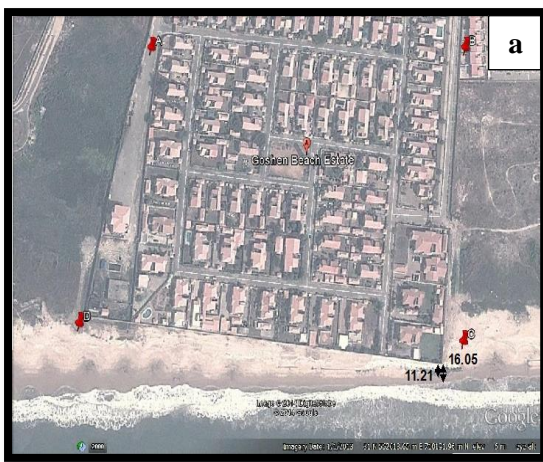
Plate 3.1a, b. Goshen Estate in 2012 and 2013 showing distances of the fence from the coastline. Note the beach configuration before the construction of groins; a. Goshen Estate in 2012 showing distance of fence from the coastline -19.63m & wet/dry line - 14.80m; b. in 2013 showing distance of fence from coastline – 16.05m & wet/dry line – 11.21m (after erosion/ocean surge of July 2012 (Imagery source: Google Earth, 2012 & 2013).
