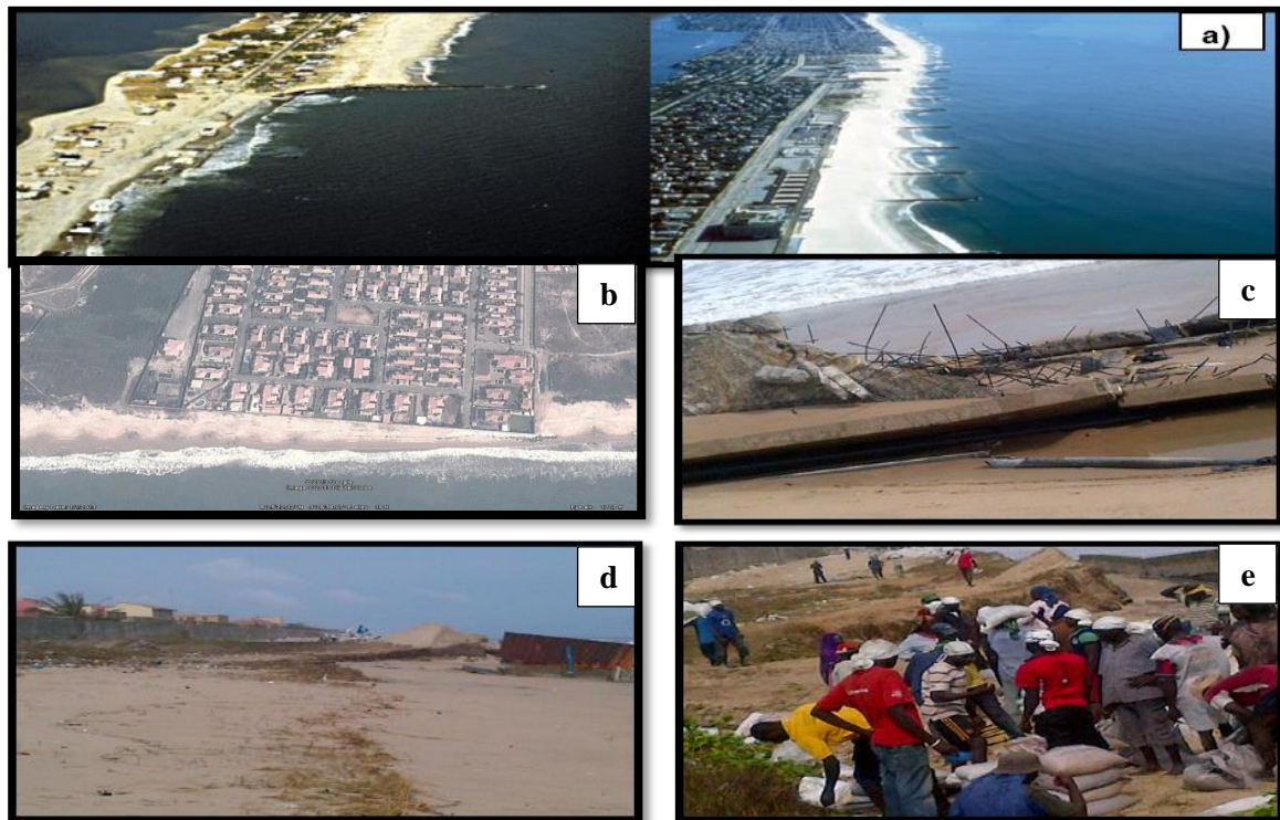
Plate 1.1a – e: Beach erosion and devastation on barrier island coastlines. a) Beach Erosion and deposition are regular features of barrier island coastlines. Groins interrupt the natural sand flow and can exacerbate erosion on downdrift side of the coastline. (Source: Tanski, 2007). b) 2013 imagery showing erosion around Goshen Beach Estate, Lekki (source: Google Earth, 2013). c) Goshen Beach Estate - remains of shallow-depth retaining wall after the ocean surge of 24-8-12, d & e- Goshen Beach Estate - devastation from the surge of 24-8-12 & workers readying sandbags as barriers to ocean surge.
