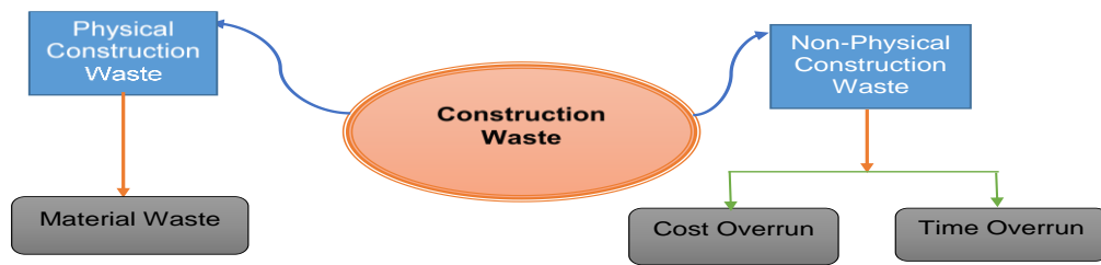
Figure 1: Classification of Construction Waste
